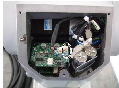
4. Remove the control board 1.
