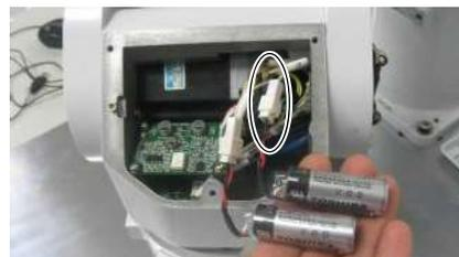
7. Bind two batteries to the plate using a wire tie.
