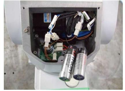
Set the wire tie on the groove of the plate.
