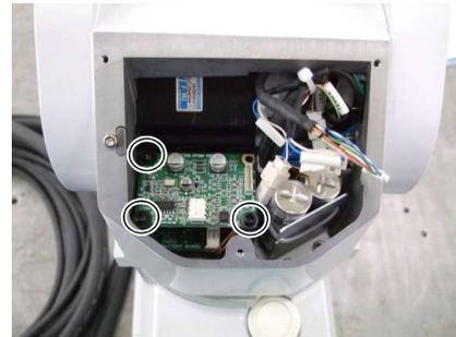
5. Disconnect the three connectors from the battery board.
