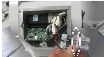
5. Disconnect the connector of one of two batteries. Then, connect the connector of the new battery.
