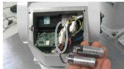
6. Disconnect the connector of the other battery. Then, connect the connector of the new battery.
