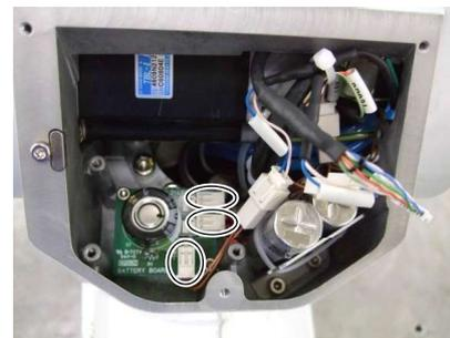
6. Remove the battery board fixed to the Arm #1.
